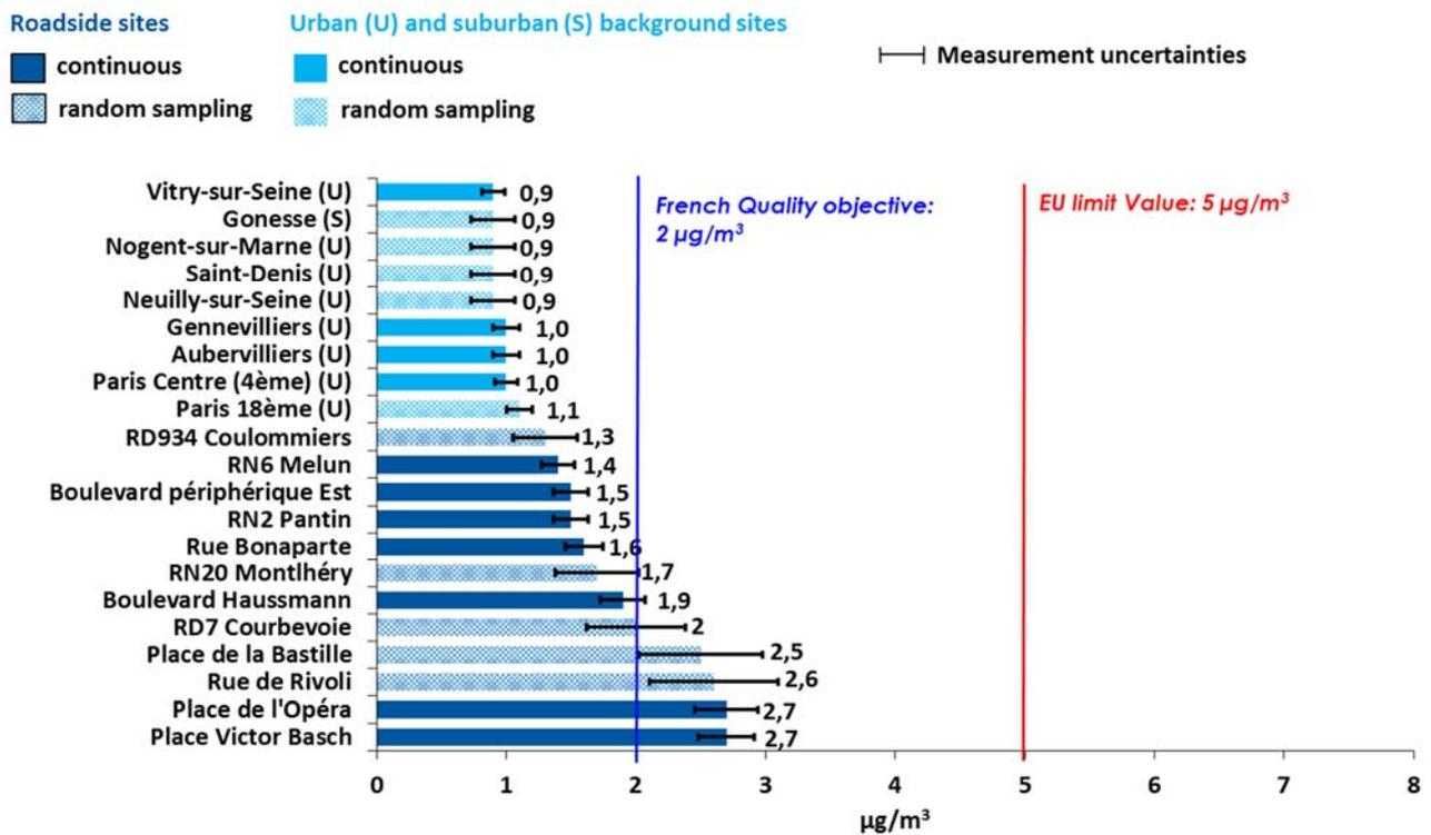
In addition to continuous measurements of benzene, discontinuous measurements are performed by AIRPARIF since 2007. These measurements are carried out using passive diffusion tubes during 12 uncontinuous weeks evenly distributed over the year. All these sites are characterised by a high pedestrian density and the presence of residences near road axes. For the random sampling sites, the results reported in this figure represent the average of twelve-weeks measurements.
