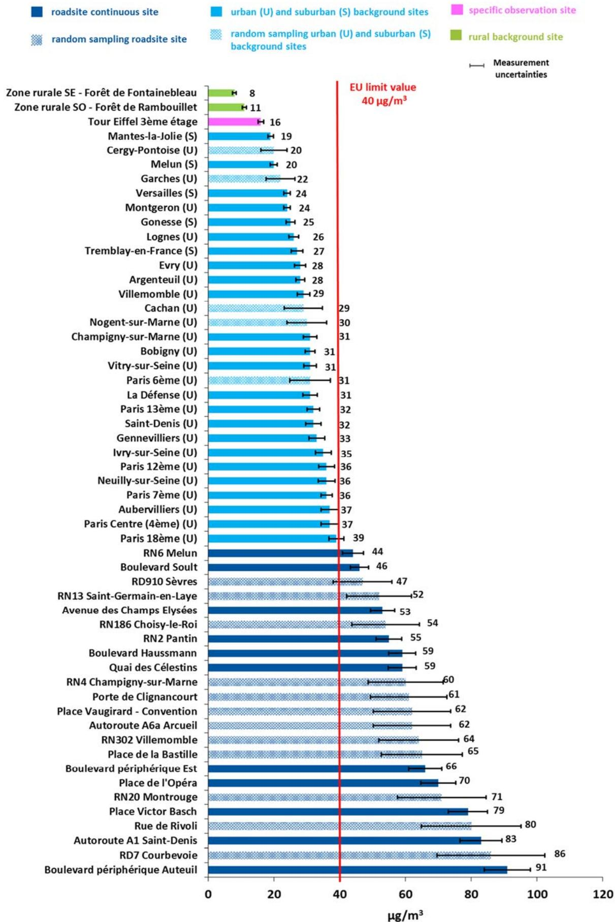
In addition to continuous measurements of NO<sub>2</sub>, discontinuous measurements are performed by AIRPARIF since 2007. These measurements are carried out using passive diffusion tubes during 12 uncontinuous weeks evenly distributed over the year. For these random sampling sites, the results reported in this figure represent the average of twelve-weeks measurements.
